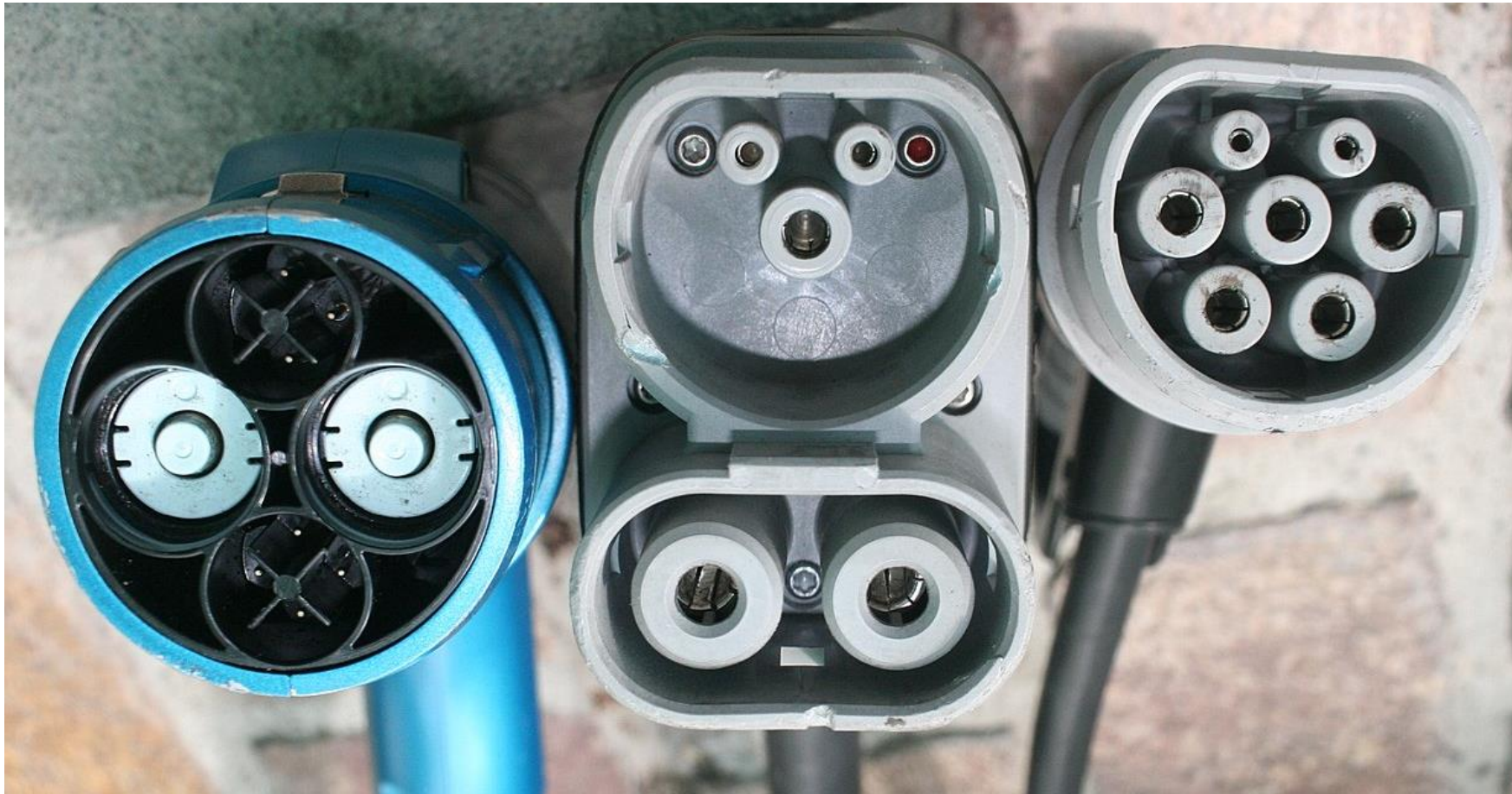
CHAdeMO (IEC 62196 type 4, DC), IEC 62196 combo2 (DC only), and IEC 62196 type 2 (AC)
